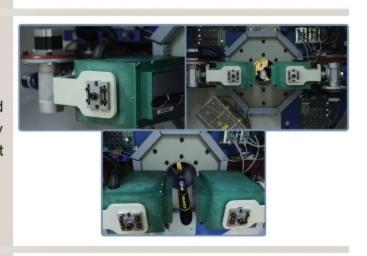
Detector module including pixelated crystal, PMT and FEE Power supply
