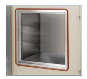
Yaran Vacuum Ovens are equipped with silicon gaskets. These gaskets resist a wide variety of temperatures and pressures. However, for solvent applications we recommend using the Buna M gaskets, and for acidic applications the Fluorosilicone gaskets due to special working circumstances.
