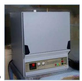
system with proper sealing could be utilized. Working temperature of up to 1250, 1450, 1600, 1700 and 1800°C are available.
