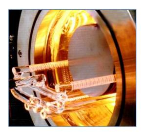
The Thermal Evaporation Process Chamber Vacuum System is capable of pumping a clean Thermal Evaporation Process Chamber to a level of <2x10E-8 Torr at room temperature with no gas flows after a 24-hour bake out. For a clean, baked-out chamber, loaded with a clean, baked-out Silicon wafer, and no gas flow, the pressure rise during heating will remain at <2x10E-7 Torr .
