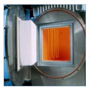
Other possibilities include the heat treatments of metals, crystal growing and the manufacturing of ceramic powders. Hydrogen processes are limited to 1000°C. Vacuum operation is only recommended in low vacuum ranges.
