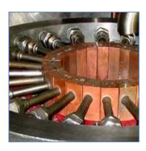
**Skull melting** is an induction melting method for metallic materials that is used to melt highly reactive metals such as titanium. No molten metal ever comes into contact with the cooled copper walls (crucible) and the whole process takes place under an inert atmosphere.
